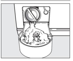
Slowly and carefully unscrew the drain filter to let the water out. Be careful not to release too much water at once. If the flow of water is too strong, some water can seep into the washing machine base and activate the water protection float switch. This will prevent the washing machine from functioning.  Tighten the drain filter back up again if you need to interrupt the flow of water.
